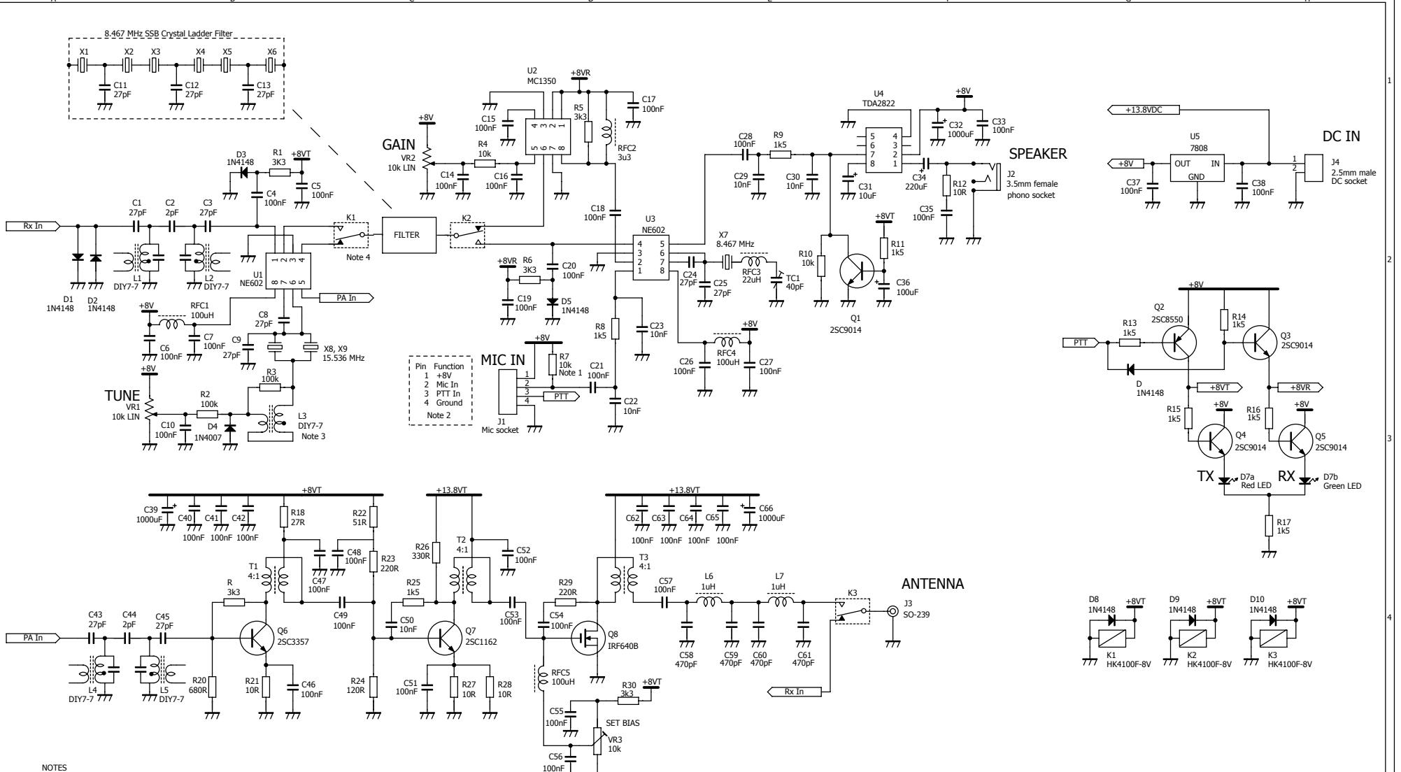
KN-Q7 40m QRP SSB Transceiver
