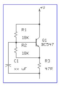
This circuit is one transistor gyrator circuit which can be easily adjusted to simulate different inductance coils just by changing the value of capacitor C2. The value of inductance the circuit simulates is approximally simulates has value of 1 henry for every 2 microfarads in C2. So if you want to make 5 henry coil simulator, you just use 10 uF electrolytic.
