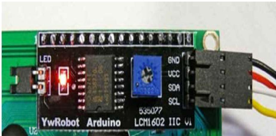
Figure 1. The back of the I2C LCD display
