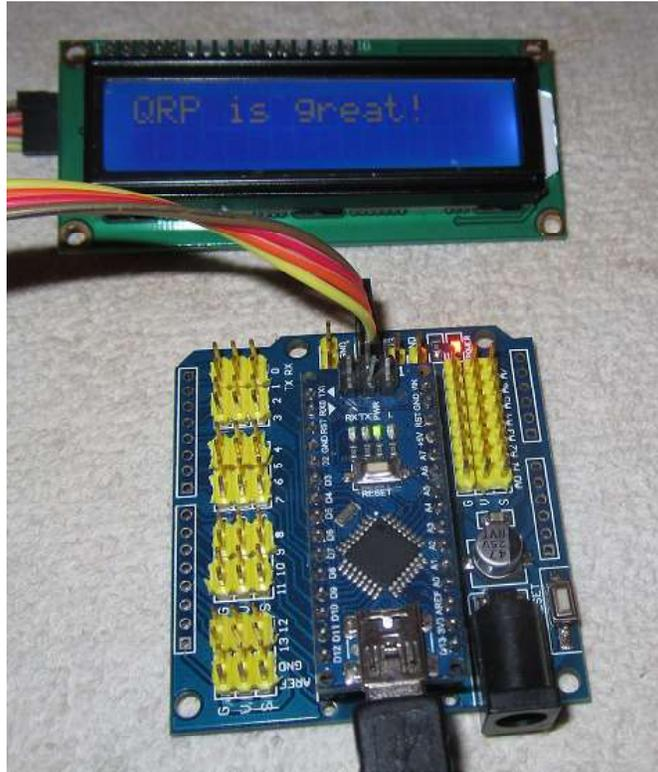
Figure 4. LCD and Nano prototype board
