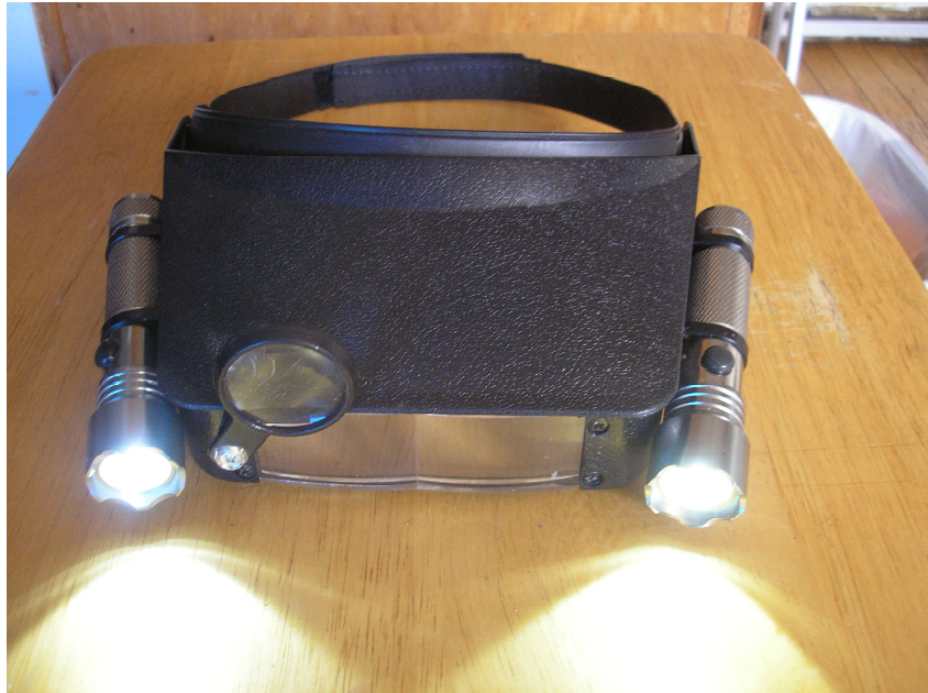
Fig. 1 Harbor Freight Headband Magnifier as modified
