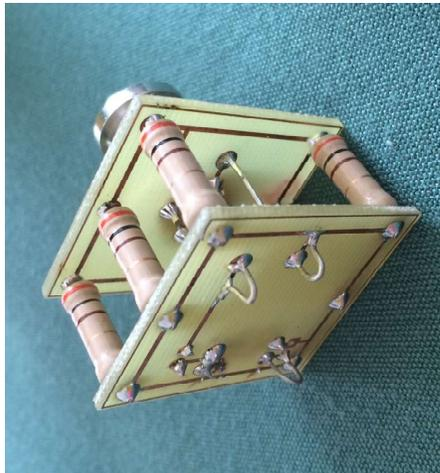
**Prototype for Pacificon Dummy Load Kit.
