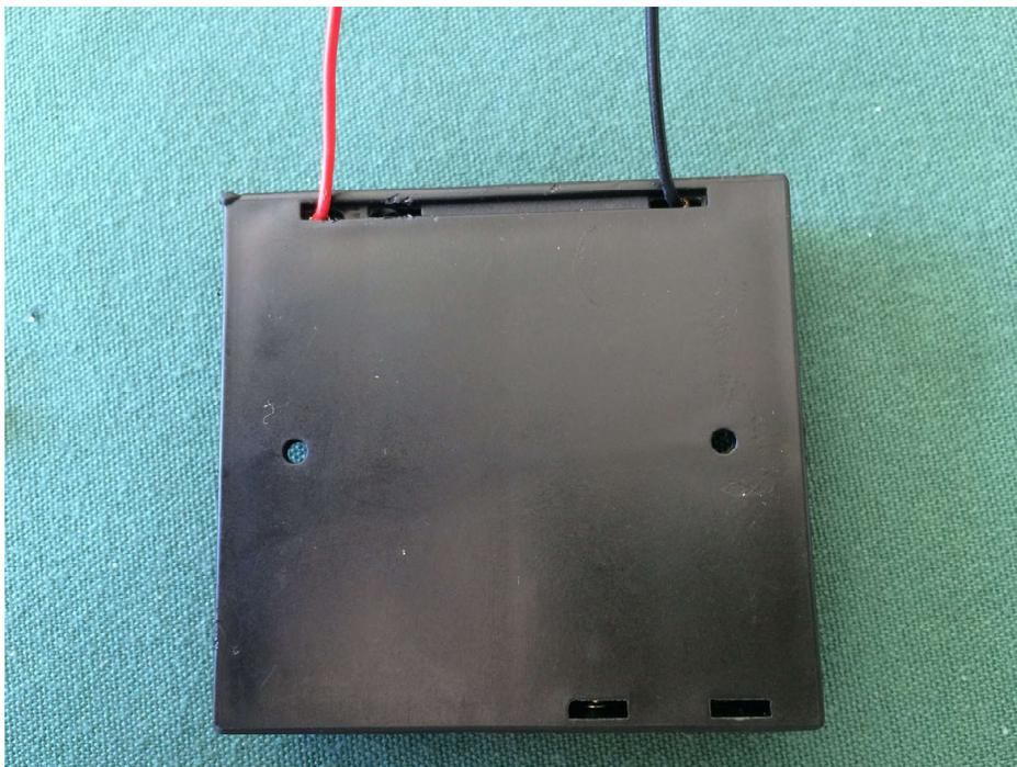
Fig. 3, Battery holder with wires rerouted.
