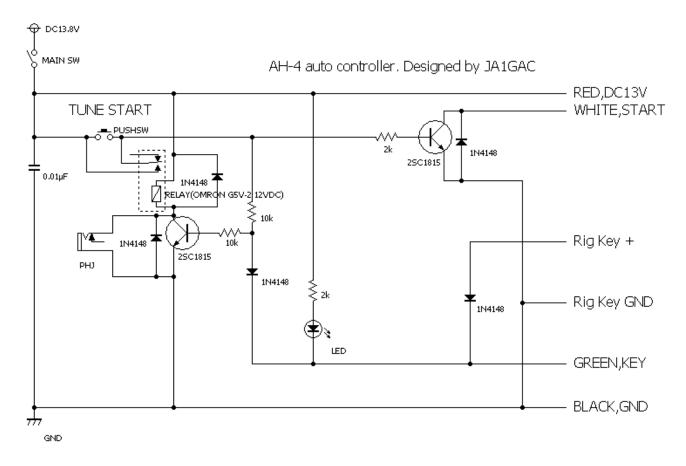
By using this circuit, tuning is achieved by pushing the start switch once shortly. And the radiation power from antenna is suppressed to only 0.3W specified by AH-4 because the transmission of carrier is started at the request of AH-4. So, you don't need to worry about affecting to other stations working in band.
