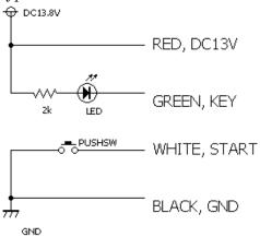
These conventional controllers are very easy to make. But for operation, following manual processes are required.
